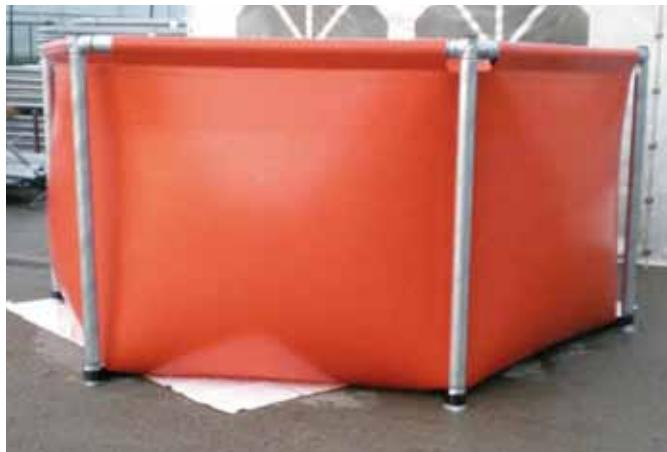
RCY Containment basins with frame work have a galvanized steel frame work, bringing resistance and strength. In the case of deterioration, the membrane can be replaced. Made in PVC, Polyurethane and specialty polymers, the fabric assures an excellent resistance for most of chemical products.
