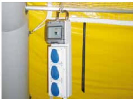
*The lighting includes a double neon light 2 x 36W, able to light up a 15m<sup>2</sup> inflatable tent. Several electrical power stations can be connected in series for the bigger surface area tent (30 to 75 m<sup>2</sup>). The power station is fixed on the top of the inflatable archs by a small chain equipped with S-hook. The electrical power station includes :*
